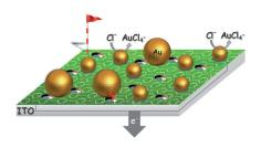
Suitable refills: Gold nanoparticles transferred together with monolayers of polyaniline onto a conducting substrate can be electro-oxidized leaving behind cavities of uniform size in the polymer films. The cavities show size-exclusion properties and the films can be used as an analytical tool for the recognition of nanoparticles.
